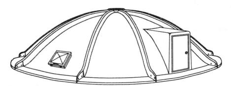
FRP is most advantageous in meeting structural requirements in hostile environments. SynTechnics free-spanning domes are structurally designed to handle appropriate live, wind, and unbalanced loading conditions. Various accessories such as windows, duct connections, vents, personnel doors and equipment hatches are readily available, sized to meet operating conditions.
